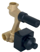
PROJECT LINE - Concealed bath shower valve with Ø35 mm ceramic cartridge, automatic diverter and 1/2" connectors. Flow rate at 3 bar: 20 l/min bath, 18 l/min shower.
